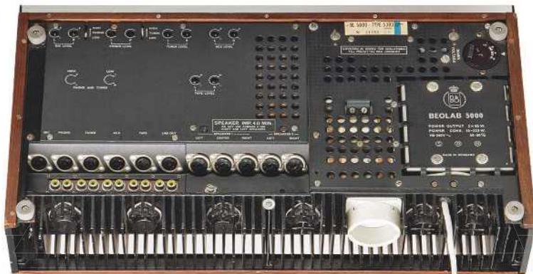
ABOVE: In this view the large heat sink for the power amplifier (left) and power supply regulator (right) can be seen. The white socket provides power for the tuner
